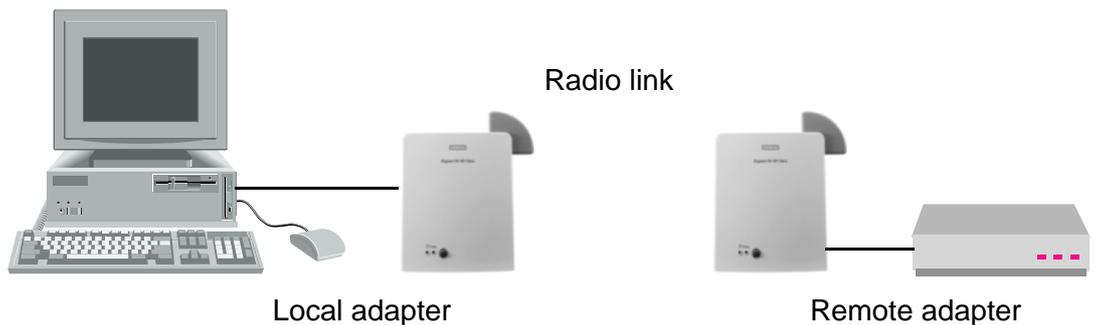
The connection between the PC and the peripheral device is routed via the radio link between the local adapter and the remote adapter.
