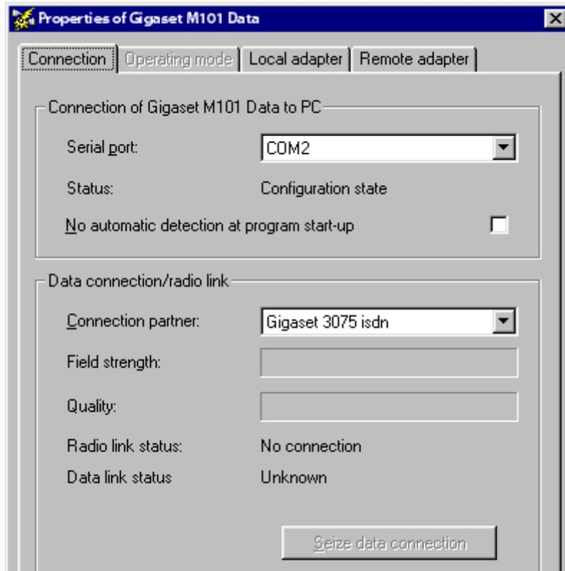
We recommend leaving the option **No automatic detection at program start-up** deactivated (as shown). The program then checks the existing COM ports and determines where the adapter is connected. Manual interface selection is only recommended if there is more than one Gigaset M101 Data unit connected to the PC.
