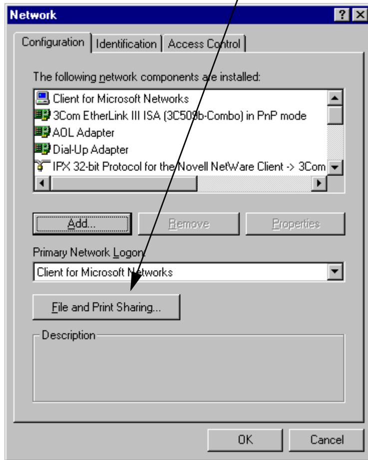
Set the parameters here. If a change was made, new drivers are loaded and Windows must be restarted.
