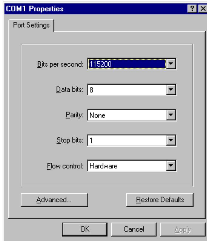
The baud rate (max. 115200) and HW handshake (default setting) are set in this mask. If you can now transfer data from one PC to another, proceed with the second step.
