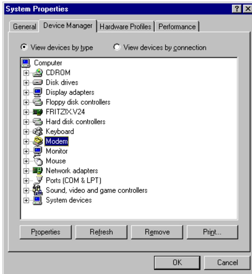
Double-click the icon to expand the branch. The setting **Null-Modem Cable at COMx** should be available. Select the appropriate COM port for your configuration and double-click it to open another subfolder.
