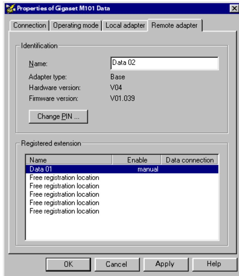
The **Remote adapter** tab is only available after registration on the **Local adapter** tab.
