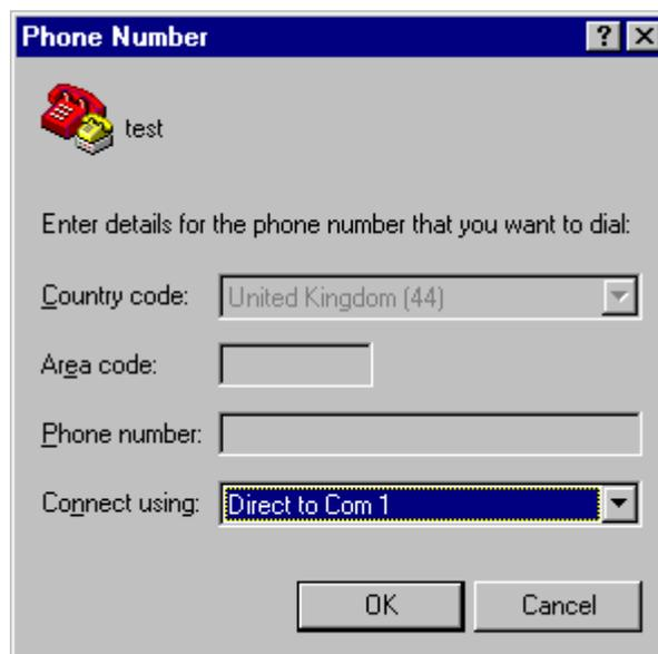
Set up a direct connection via COMx (COM 1 was selected in the example).
