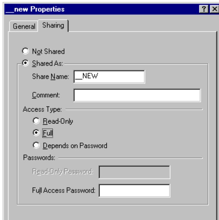
Assign the other PC user access rights to the files on your hard disk, or where applicable, activate password protection.
